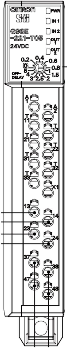
Fig. A-1: The front face of G9SE-221-T05 safety relay
