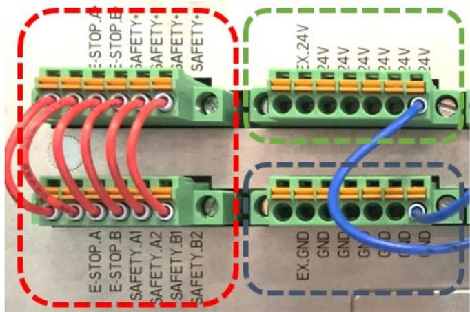
Fig. A-2: The connectors on the TM Control Box. The safety connectors are shown in red, 24 V outputs in green, and ground connection in blue.
